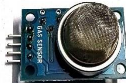
Fig. 3(f): Gas Sensor
